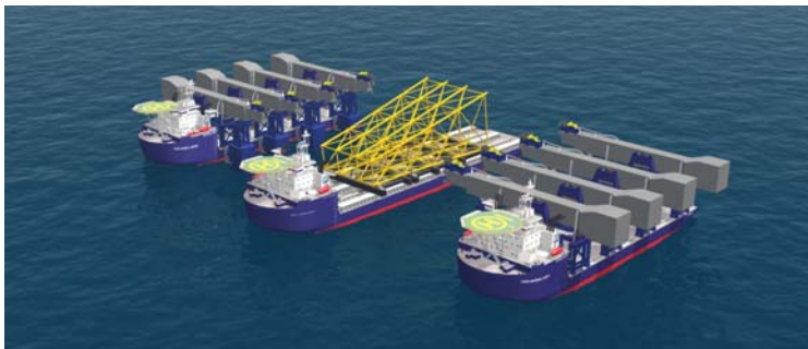
Graphic impression of Sea Metric's Twin Marine Lifter (TML) system
