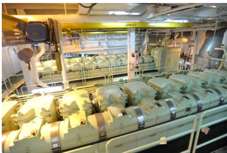
View of the engine room aboard the José María Entrecanales showing two of the MAN 9L48/60B main engines
