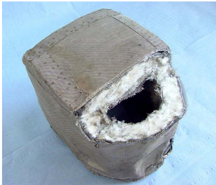
Figure 2: Covering cap cut open for evaluation of the insulation material condition (6 276 operating hours)
