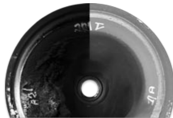
comparison of slide fuel valve before and after retrofitting
